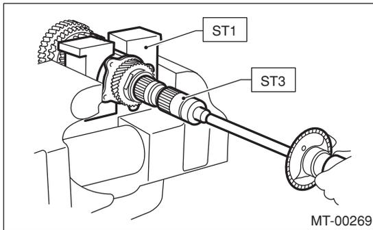
4) If the starting torque is not within the specified limit, select the adjusting washer No. 2 from following table, and recheck the starting torque.
