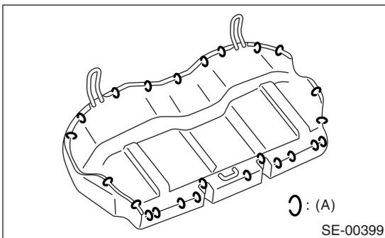
10) Remove the hog rings (A), and then remove the seat cushion cover.
