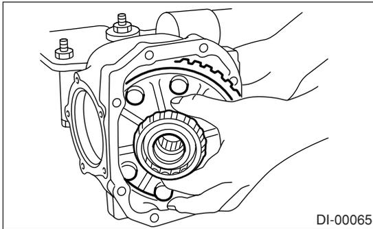
7) When replacing the side bearing, remove the bearing cup from side bearing retainer using ST.
