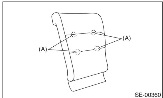
4) Remove the bolts, and then remove the backrest latch.
