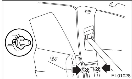
6) Remove the seat belt lower anchor bolt at center pillar lower port. (Driver's seat)
