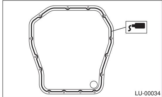
5) Tighten the bolts which install oil pan onto engine block.
