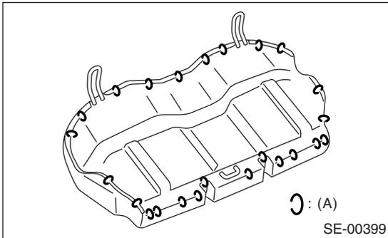
11) Remove the hog rings (A), and then remove the seat cushion cover.
