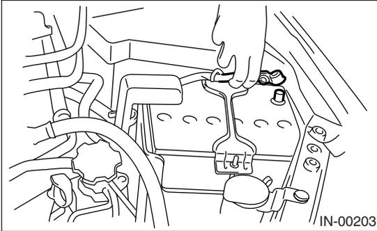
2) Disconnect the connector from tumble generator valve actuator RH.
