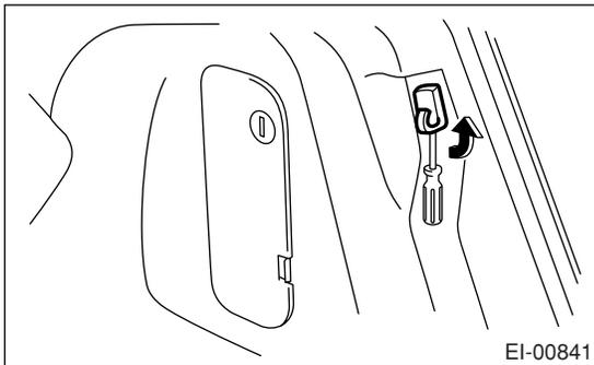
5) Remove the trim clips, and remove the trunk side trim.
