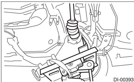
8) After inserting the rear differential stud bolt into rear crossmember bushing, lift up the transmission jack and align the rear differential with its own position.
