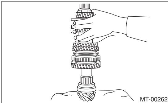
14) Install the drive pinion collar, needle bearing, adjusting washer No. 2, thrust bearing, adjusting washer No. 1 and differential bevel gear sleeve in this order.
