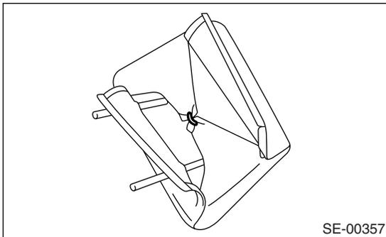
9) Remove the hog rings (A) on the rear side of seat cushion.
