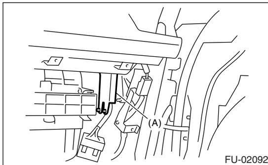
4) Disconnect the connector from main relay.
