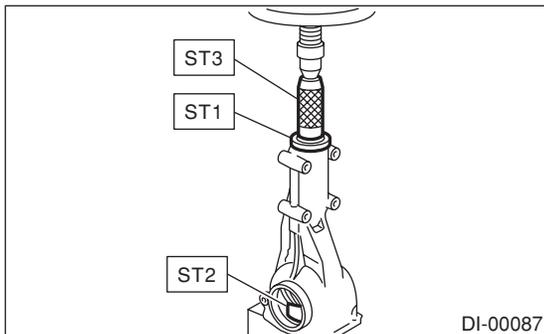
6) Insert the collar, then press-fit the pilot bearing with ST1 and ST2.
