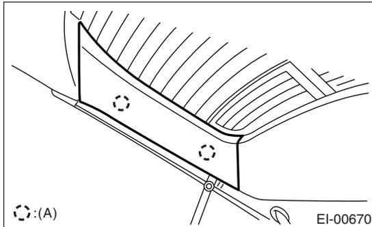
2) Remove the clips, and detach the rear gate upper trim.
