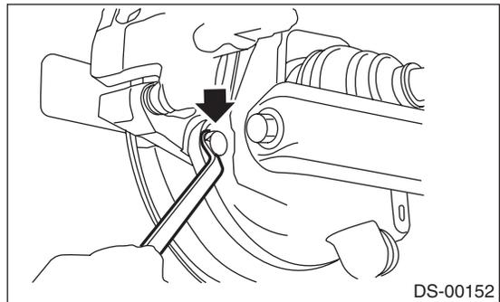
8) Install the rear ABS wheel speed sensor and brake cable bracket.
