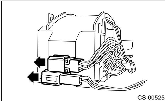
9) Remove the sheet, and remove the shift lock solenoid assembly.
