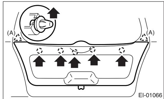
6) Remove the rear gate weather strip.
