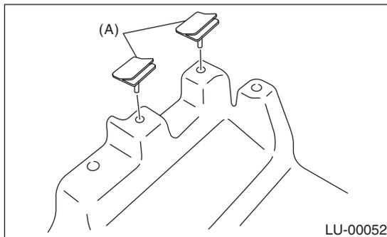
2) Install the baffle plate.
