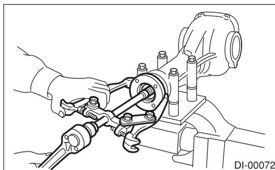
14) Press the end of drive pinion shaft and extract it together with rear bearing cone, pinion height adjusting washer and washer.
