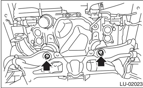
8) Install the front exhaust pipe. <Ref. to EX(H4DOTC)-6, INSTALLATION, Front Exhaust Pipe.> <Ref. to EX(H4SO)-5, INSTALLATION, Front Exhaust Pipe.>
