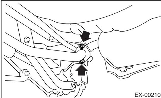
2) Remove the cushion rubbers, and detach the muffler.
