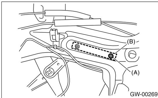
9) For glass stroke adjustment, install the ST to glass, close the door, and raise the glass with regulator until positional relationship between glass and weather strip becomes as shown. And secure the glass so that the upper stopper correctly touches the glass holder.
