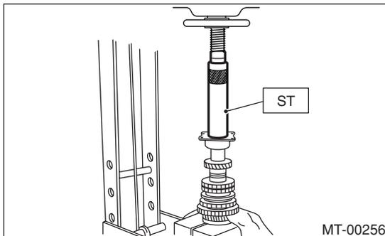
9) Position the woodruff key in groove on the rear of driven shaft. Install the 5th driven gear onto driven shaft using ST and press.
