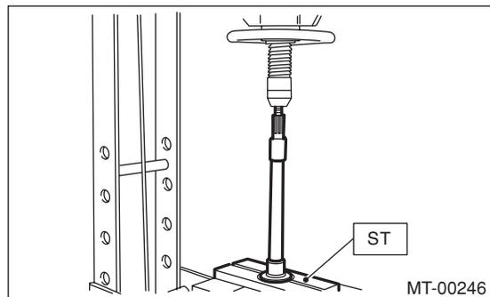
4) Unlock the caulking of lock nut. Remove the lock nut using ST1 and ST2.
