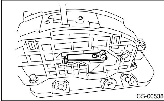
7) Remove the bolt, and separate the guide plate upper from plate lower.
