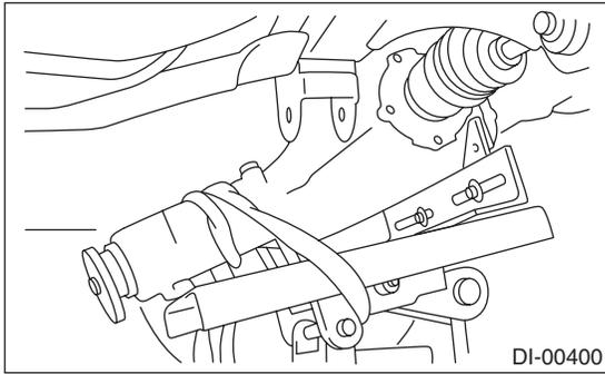
17) Lower the transmission jack stand after removing the rear differential stud bolt from rear cross-member. Rear drive shaft should not come into contact with lateral link bolt.
