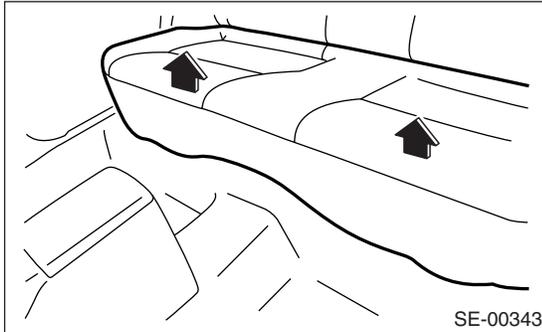
2) Remove the hook (A) by pushing it backward while lifting up the front side of seat cushion to detach seat cushion.
