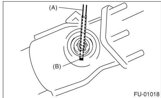
3) Install the joint pipe. <Ref. to EX(H4DOTC)-11, INSTALLATION, Joint Pipe.>
