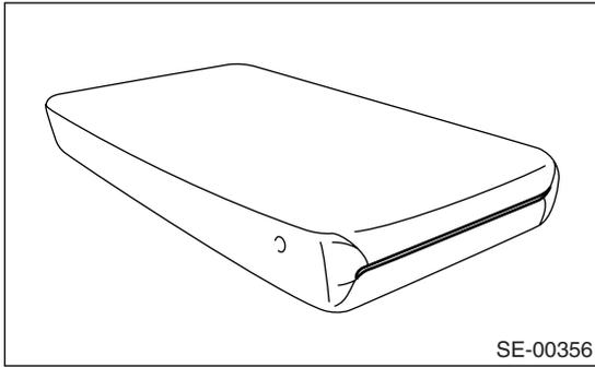
9) Remove the hook and hog ring, and then remove the headrest cover.
