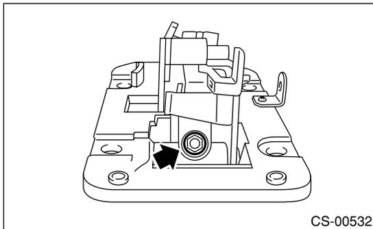
17) Remove the clamp, and remove the arm assembly and bushing plate.
