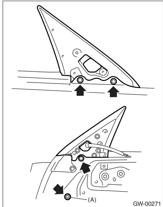
15) After adjustment, tighten the bolts and nuts.
