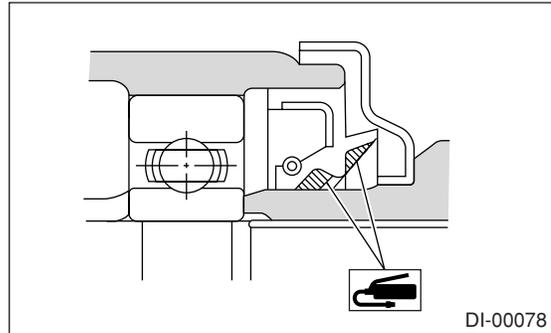
1) Adjusting preload for front and rear bearings: Adjust the bearing preload with collar and washer between front and rear bearings. Pinion height adjusting washer are not affected by this adjustment. The adjustment must be carried out without oil seal inserted.
