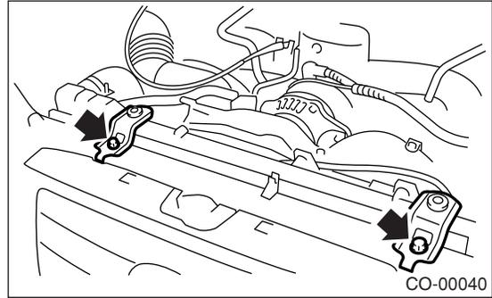
14) Install the intercooler. <Ref. to IN(H4DOTC)-12, INSTALLATION, Intercooler.>
