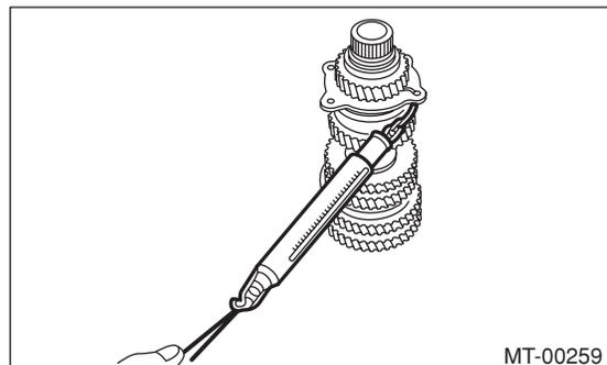
11) Install the roller bearing onto drive pinion.
