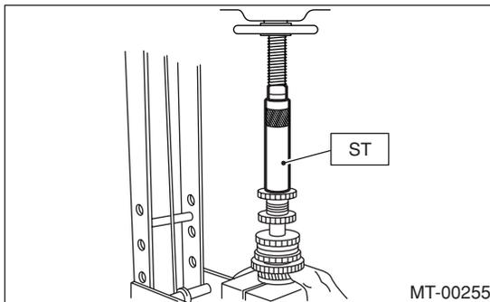
8) Install a set of roller bearings onto the driven shaft using ST and press.
