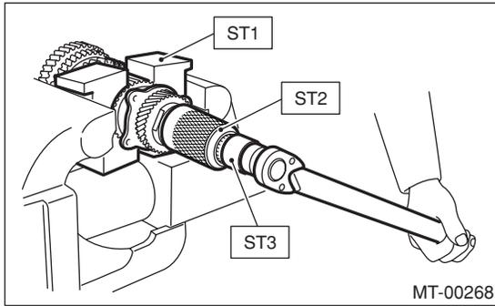
3) After removing the ST2, measure the starting torque using torque driver.
