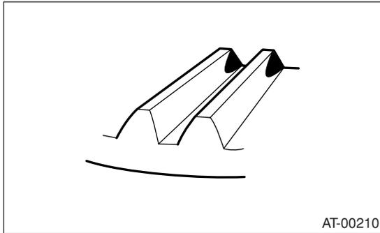
Corrective action: Reduce thickness of drive pinion height adjusting washer in order to bring drive pinion away from hypoid driven gear.
