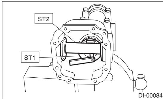
(3) Obtain the thickness of pinion height adjusting washer to be inserted from the following formula, and replace the temporarily installed washer with this one.
