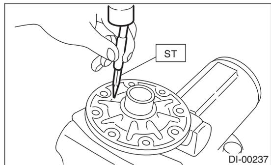
11) Draw out the pinion mate shaft and remove pinion mate gears, side gears and thrust washers. (Model without LSD)
