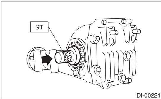
4) Install the rear differential. <Ref. to DI-29, INSTALLATION, Rear Differential (T-type).> <Ref. to DI-45, INSTALLATION, Rear Differential (VA-type).>
