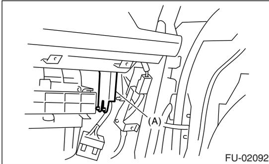
4) Disconnect the connector from electronic throttle control relay.
