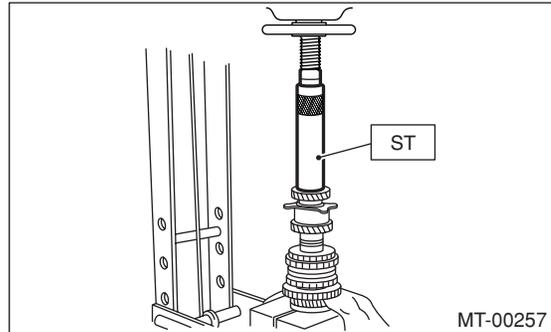
10) Install the lock washer. Install the lock nut and tighten to the specified torque using ST.
