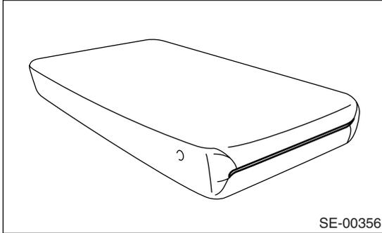
8) Remove the hook and hog ring, and then remove the headrest cover.
