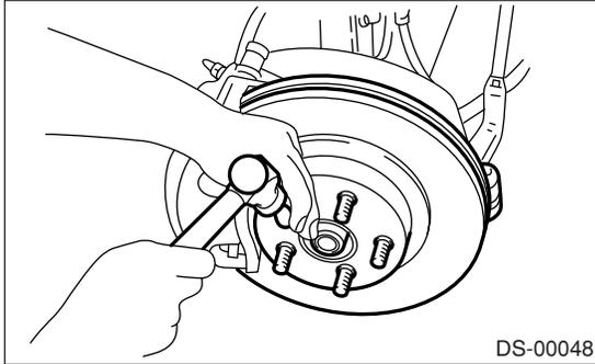
12) Install the wheel and tighten the wheel nuts to specified torque.
