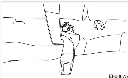
4) Remove the bolts which secure the bottom of backrest.
