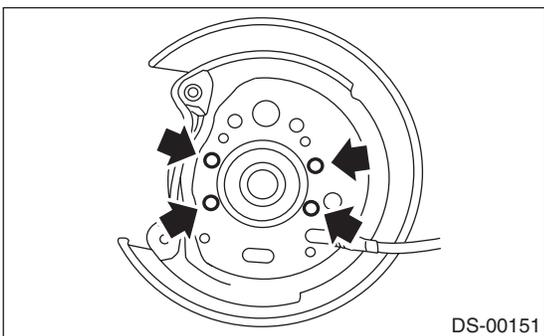
2) Tighten the four bolts to the back plate.
