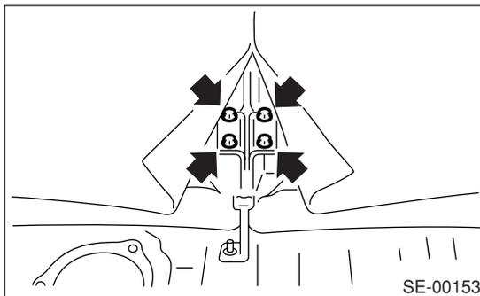
7) Remove the backrest from hinge assembly LH (hinge assembly RH).
