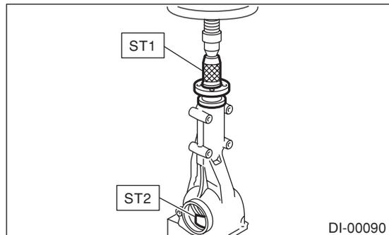
9) Install a new self-locking nut and secure the companion flange using ST and tighten the nut.
