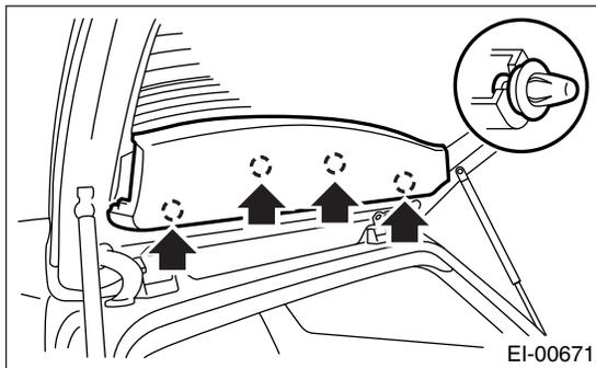
3) Remove the cover in the inner handle, loosen the inside screw.
