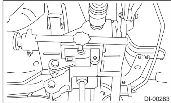
9) Tighten the rear crossmember self-locking nut temporarily.
