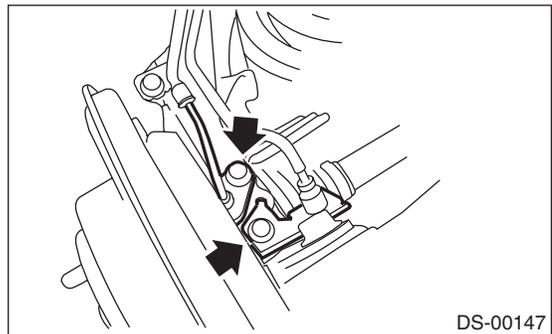
9) Adjust the parking brake lever stroke by turning adjuster. <Ref. to PB-4, ADJUSTMENT, Parking Brake Lever.>
