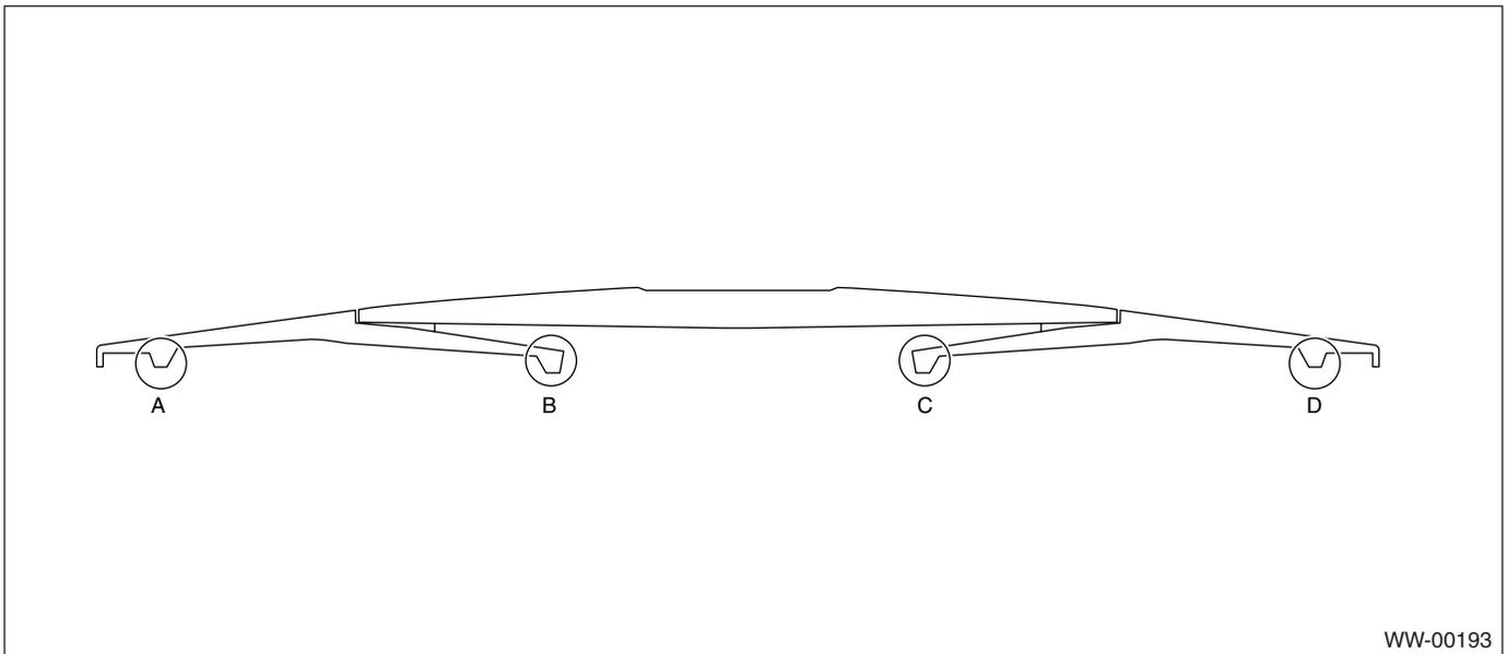
1) Insert the wiper rubber through the claw B.
