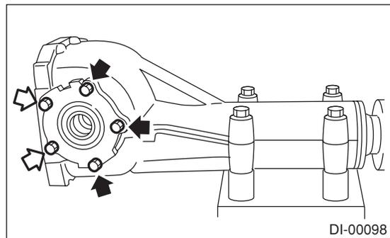
24) Install the new gasket and rear cover to the differential carrier, and tighten the bolts to specified torque.
