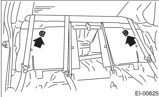
4) Insert the flat tip driver from the lower side of trunk hook, and then remove the trunk hook with rotating it 90°.
