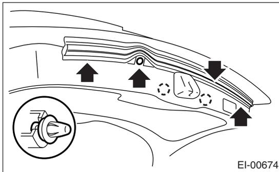
5) Remove the clips (A), remove the rear gate lower trim.
