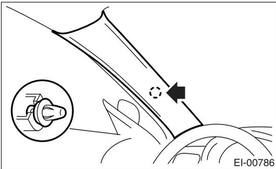
3) Remove the front inside scuff plate, rear inside scuff plate and center pillar lower trim. <Ref. to EI-60, REMOVAL, Lower Inner Trim.>
