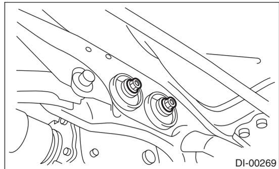
10) Remove the band from rear differential. Lift up the rear differential until the rear differential is separated from the transmission jack.
