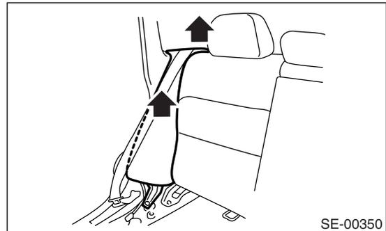
10) Remove the belt cover (A) from backrest shoulder cover, and then pull out the seat belt.
