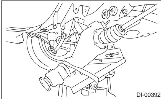
18) Pull out the axle shaft from rear differential.
