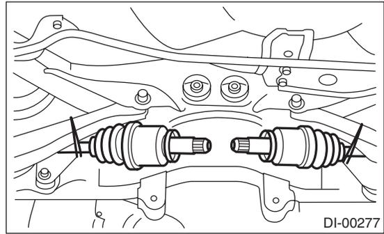
21) Remove the rear differential member plate from rear differential.
