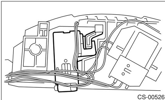
10) Remove the switch assembly.
