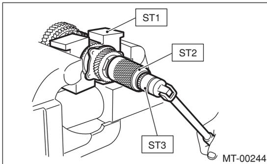
2) Draw out the drive pinion from driven shaft.
