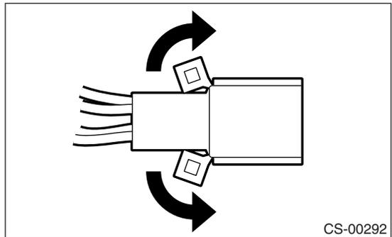
13) Disconnect the terminals of SPORT mode switch and shift lock solenoid assembly from connector, using a flat-tip screwdriver with thin tip.
