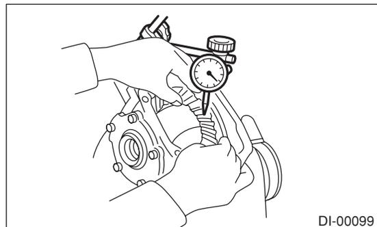
16) Check the hypoid driven gear runout on its back surface, and make sure that pinion and hypoid driven gear rotates smoothly. If the hypoid driven gear runout on its back surface exceed the specification, verify that there is any foreign material between hypoid driven gear and differential case, and they are not deformed.
