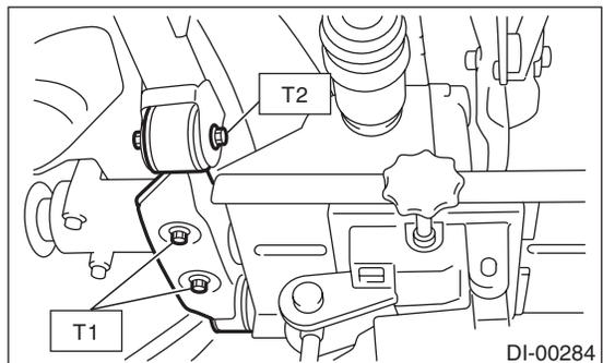
12) Tighten the self-locking nut.
