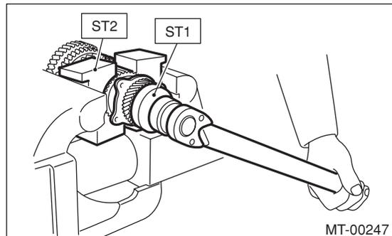
5) Remove the 5th driven gear using ST.
