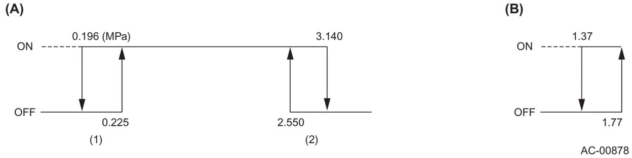
**(A)** High and low pressure switch
