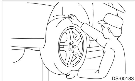
2) Inspect the lean of axis direction using a dial gauge. Replace the hub bearing if the lean range exceed the limitation.
